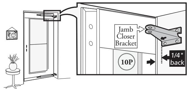
*Note: Removing the door jamb bracket from the closer may make this installation of the bracket easier.*
