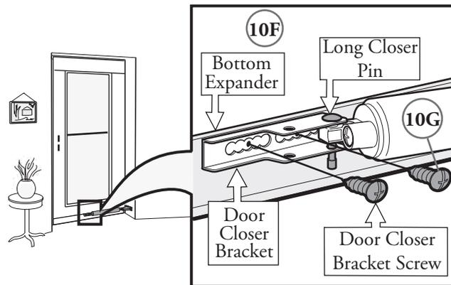
H. **Measure the distance from the hinge side of the entryway**, to the end of the bottom door closer bracket. Mark this end distance approximately 2" from the top of the door.
