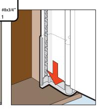
**5E** Pre-drill and install inside jamb screws through the inner side of the hinge rail in all 6 remaining locations. Do not over tighten screws.
