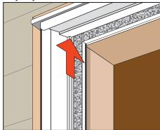
**7E** Starting at the top hole, pre-drill and fasten the latch rail with a #6x1" mounting frame screw. Ensure there is a consistent reveal between the door and latch rail. Continuing down the latch rail, pre-drill and install one mounting frame screw at a time, keeping a consistent reveal.
