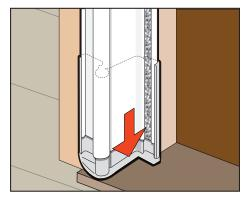
**7F** Cut rail extender weather stripping to length, peel adhesive backing and install.
